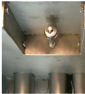
Upper float switch.
