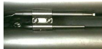
High-limit (upper) and temp probe in cook vessel.
